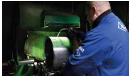
Magnetic particle inspection
